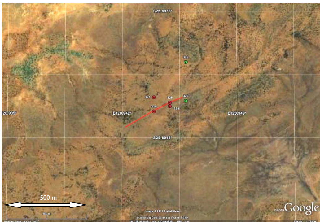
Figure 3: Manganese mineralisation zone mapped / sampled at the Shoemaker project: red dots – Mn-rich rock chip samples collected in July 2010; green dots – Fe-rich rock chip samples collected in July 2010; red line – Mn mineralisation zone outcrop and scree mapped in July 2010
