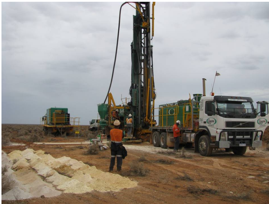
Figure 4: Pre-collar RC drilling at the Eyre project in March 2010
